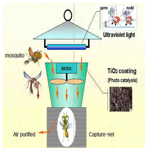
Figure for principle of new mosquito trap
