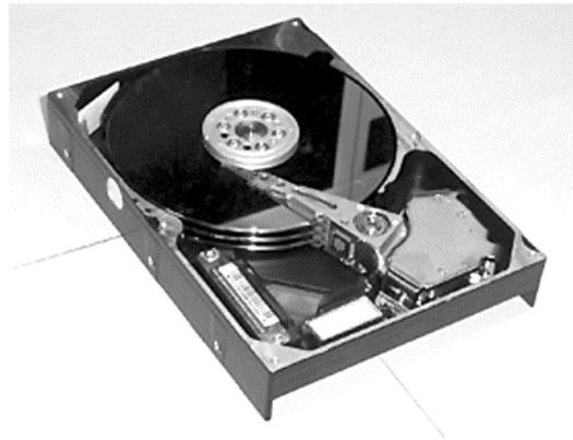
Figure 4. Image of hard drive with cover removed to reveal magnetic disk, actuator arm and read/write head
